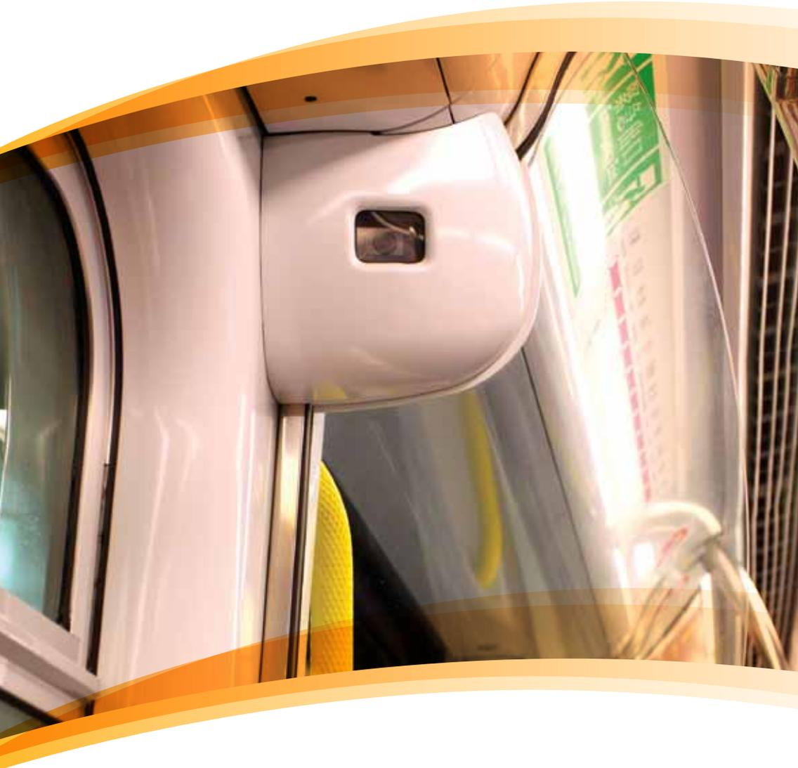
Recording quality permits evidential video to be taken from the seating and doorway areas to clearly identify offenders. Vertical infra-red detectors are situated at all vehicle doors to determine passenger flow in both directions.
