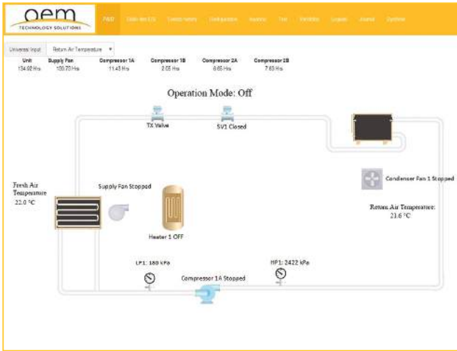
1 Circuit, 1 Compressor & 1 Heater Configuration
