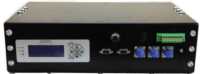
OEM's Selective Door Opening (SDO) Unit is an example of subsystem the utilises the WTCB.
